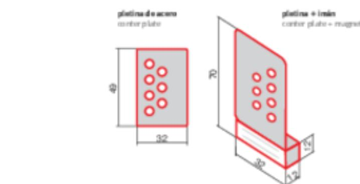
Magnetic metal supports designed to build customised manhole covers using tiling pieces from each installation. It enables easy access to piping, mechanisms and so on, meaning it remains totally integrated, invisible from the outside.
